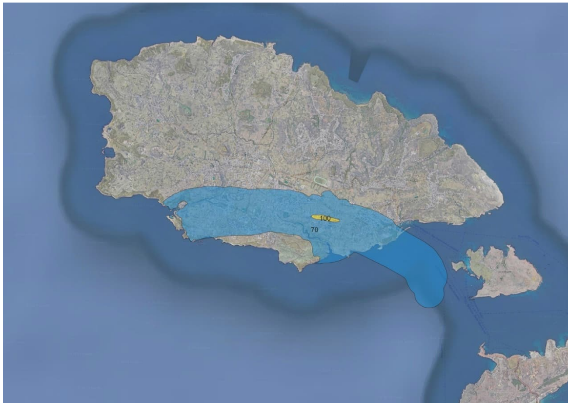
Figure 6-4 Scenario 1 single track extent of 70 dB L_{Amax} and highest L_{Amax} from scenario.
