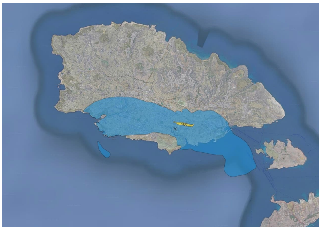
Figure 6-3 Scenario 1 with dispersed tracks, extent of 70 dB L_{Amax} and highest L_{Amax} from scenario.
