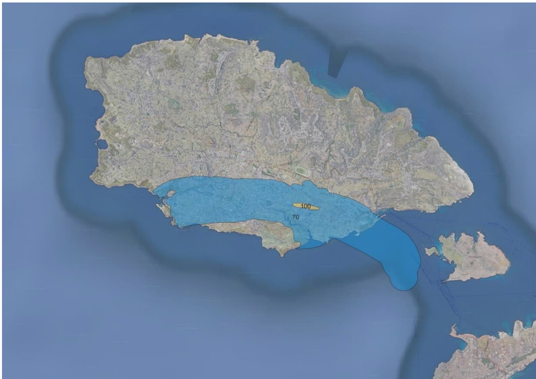
Figure 6-8 Scenario 2 single track extent of 70 dB L_{Amax} and highest L_{Amax} from scenario.
